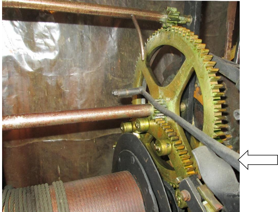
Picture 3. The brass drive wheel with one of the strike rollers about to activate the micro-switch. The black iron rod seen at an angle (arrowed) stops the strike mechanism after the required number of strikes.
