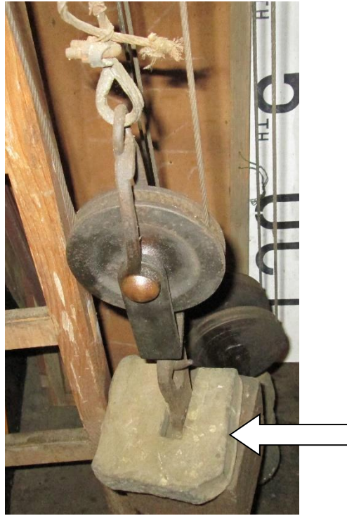
Picture 5. One of two weight blocks suspended by wire and pulley wheels; this block powers the 'Strike Train' and is made from cast iron and has an extra weight (arrowed) of lead probably to overcome increased friction in the weight system due to age. The other weight block powers the 'Going (Time) Train' and is cylindrical and made of lead, also with an added lead weight.
