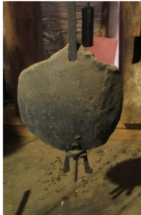
Picture 9. The lead pendulum showing the adjustment screw (arrowed).
